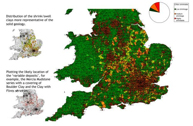
Here we have plotted valid claims from a large sample (around 80,000) to illustrate the significance of the geology. Low shrinkage clay soils are shaded dark green. The lighter shades of green, orange and red show the highly shrinkable soils as defined above.
