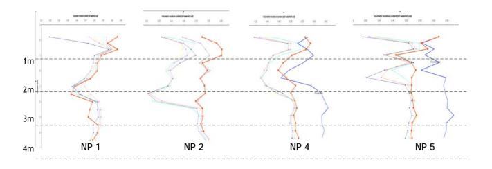
For reference purposes, Station NP 1 is nearest to the tree and NP 5 furthest away. We have omitted the readings from NP 3 due to the variable geology (gravel, sands and clay) and the relatively shallow depth of the bore.
