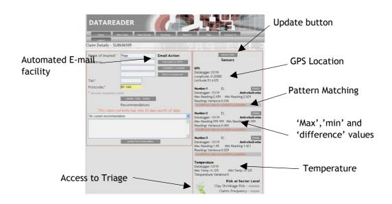
The temperature is also recorded, along with the minimum, maximum and 'difference' values. We can see very quickly which parts of the building are moving and which soils are drying more than others.
